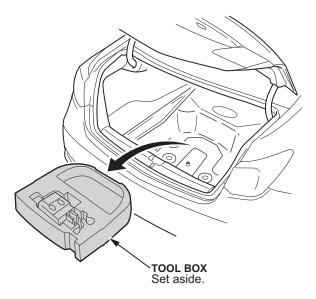
6. Install the jack, the wheel nut wrench/jack handle, and the extension bar into the new tool box.
