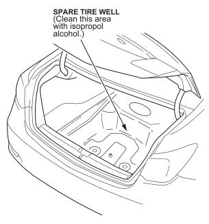
8. Remove the adhesive backing, and install the spare tire cover with the arrow pointing to the front of the vehicle.
